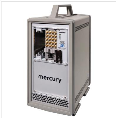
**The 8257A is a low-cost, SOSA aligned 3U VPX chassis ideal for developing applications on Mercury's SOSA aligned 3U VPX boards.\*** Providing the required power and cooling in a small desktop footprint, the chassis allows access to all required interfaces on these boards without the need for a larger, more expensive multi-slot chassis.
